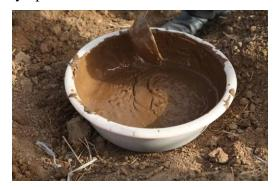
5. Insert the sensor into the hole and rotate the sensor left and right to distribute the mud evenly around the sensor.
