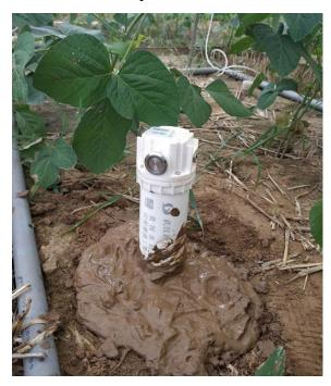
The purpose of grouting: to make the installed integrated moisture meter and the soil more closely and seamlessly, so as to ensure more accurate measurement data. Because the water content of the grouting mud is higher than the actual soil water content, the automatic measurement data can only be used after the grouting is basically solidified after one to two days.
